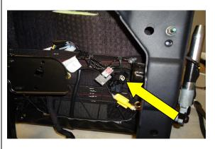
STEP 11: CONNECT THE SEAT BELT SENSOR DEVICE TO THE CABLES AND USING ZIP TIES ATTACH THE LOOSE CABLES TO THE SEAT.
