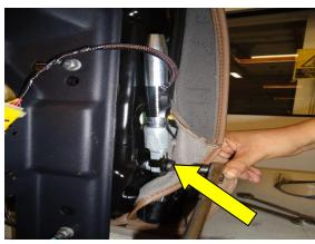
STEP 3: DISCONNECT ALL OTHER CABLES AND UNBOLT THE SEAT BELT SENSOR DEVICE AND PLACE IT TO THE SIDE.
