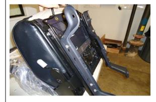
STEP 8: PLACE THE ADJUSTERS ONTO THE MASTERCRAFT SEAT AND HAND TIGHTEN NUTS.
