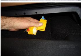
STEP 2: DISCONNECT THE SEAT BELT SENSOR UNDER THE SEAT BEFORE REMOVING SEAT FROM VEHICLE.
