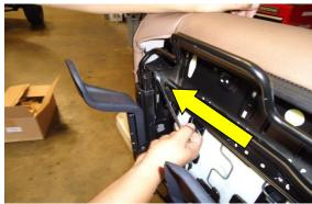
STEP 4: MOVE ADJUSTERS TO THE REAR POSITION AND UNBOLT THE (2) FRONT ADJUSTER NUTS. RETAIN THE NUTS FOR LATER USE.
