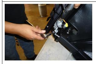
STEP 9: AFTER TIGHTENING ADJUSTERS, INSTALL THE SEAT BELT SENSOR DEVICE USING THE 7/16" X 1-1/4" BOLT SUPPLIED IN THE KIT.
