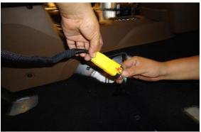
STEP 12: PLACE SEAT IN VEHICLE AND LINE UP MOUNTING HOLES TO MOUNTS AND CONNECT THE SENSOR CABLES.
